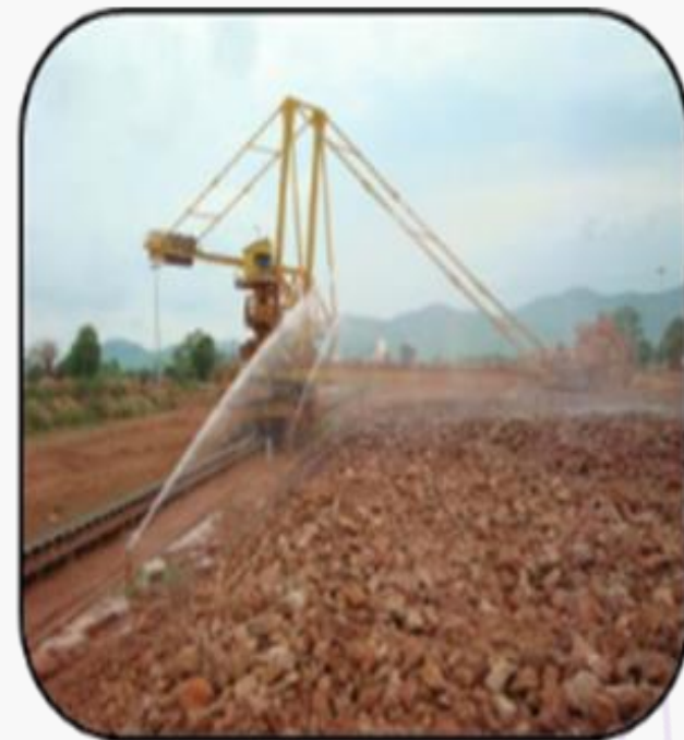
Water sprinklers at bauxite handling
